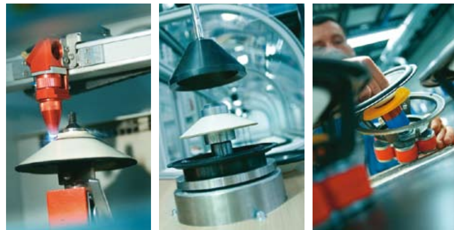
The W composite sandwich is made of a very rigid foam core, covered on each side by glass fabric skins.
